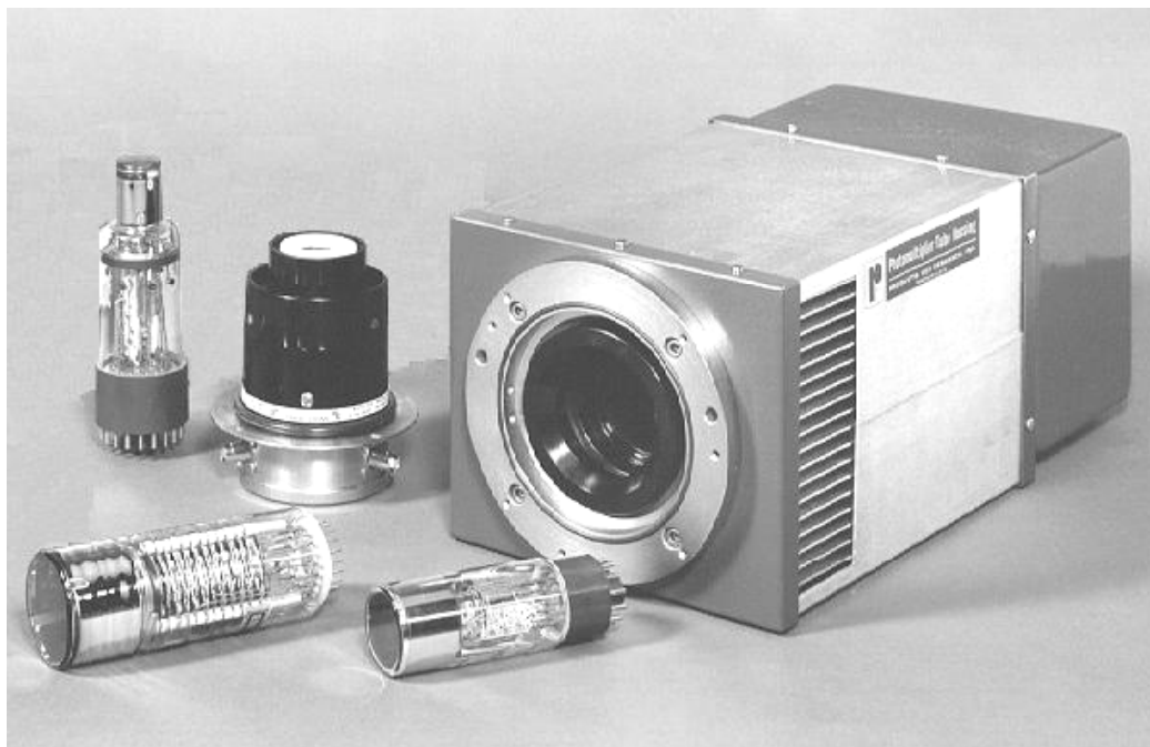
Fig.(2) :Photograph showing Cooled Photomultiplier Housings for PMT EMI 9863Q [1].
