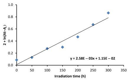
Fig.(4): Changes in  $ln(A_t - A_{\infty})$  for PVC film containing  $Me_2SnL_2$  with irradiation time.
