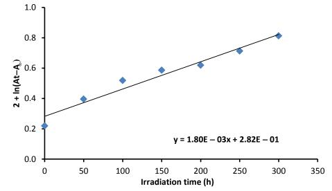
Fig.(6): Changes in  $ln(A_t - A_{\infty})$  for PVC film containing Ph<sub>3</sub>SnL with irradiation time.
