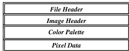
Structure of 8-bits BMP file
