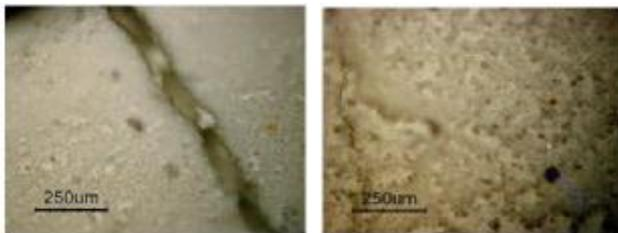
Fig. (4) Micrographs of 90%HA+10%PSZ layer produced by EPD on Ti-20Co alloy.
