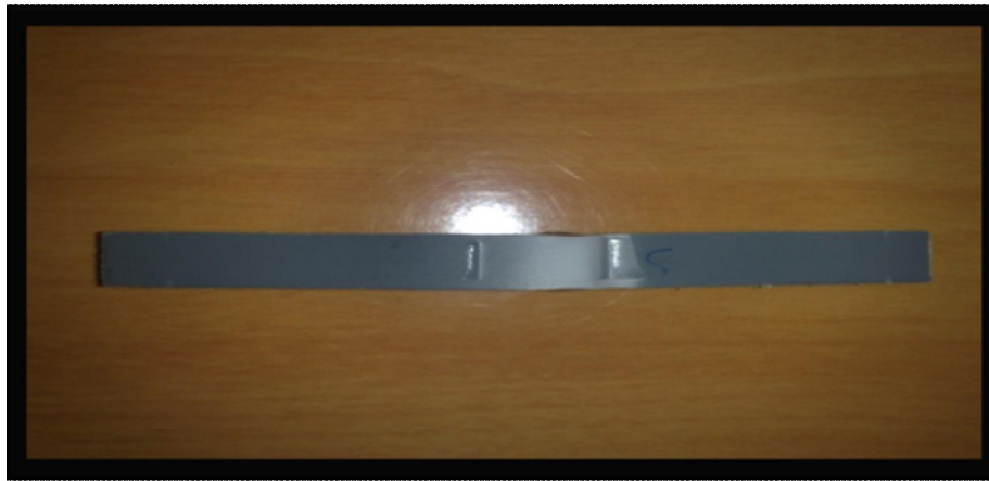
Fig.(3) Flexural test specimen after final failure.
