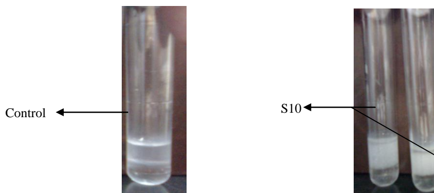
Fig. (2) The emulsification index (E24%) for S10 (the supernatant of culture media were added with kerosene and left at room temperature for 24 hrs.).
