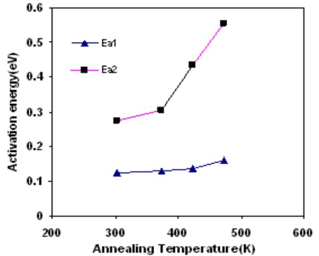
**Fig.(3) Variation of activation energy with annealing temperature.**
