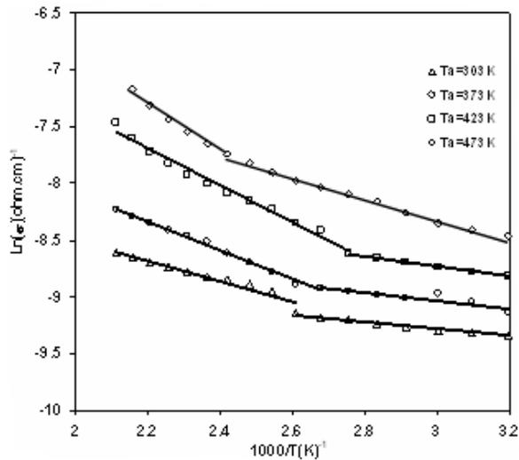
**Fig.(2) Dependence of  $\ln\sigma$  on temperature for different annealing thin CdTe films.**
