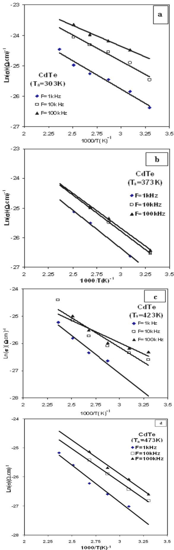
Fig.(4) The relation between  $\text{Ln} \sigma_{ac}$  vs.  $1000/T$  for as deposited and annealed films.
