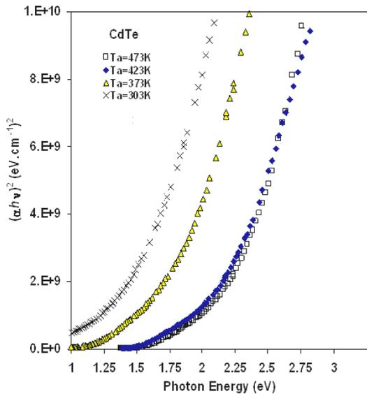
**Fig.(6) The relation between  $(\alpha h\nu)^2$  and photon energy  $(h\nu)$  for annealed and un-annealed CdTe thin films.**
