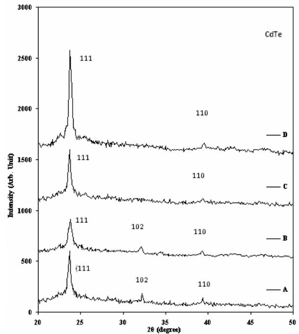
**Fig.(1) X-ray diffraction pattern for films (A) as-deposited (B)  $T_a=373$  K (C)  $T_a=423$  K (D)  $T_a=473$  K.**
