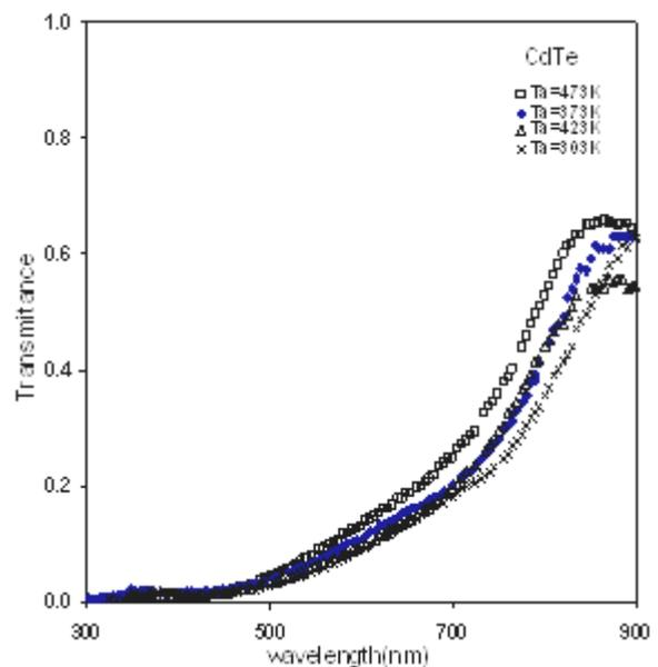
Fig.(5) The transmittance spectra for annealed and un-annealed CdTe thin films.
