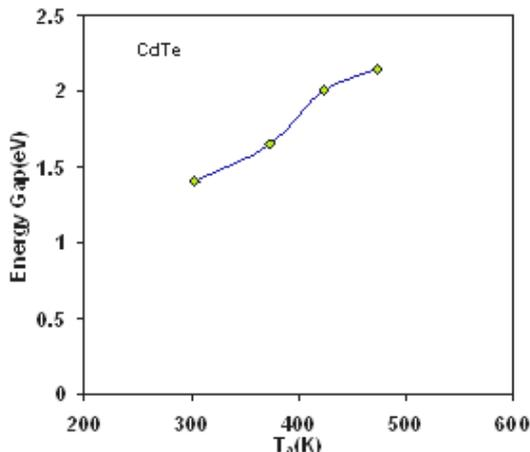
**Fig.(7) Variation of energy gap with annealing temperature.**
