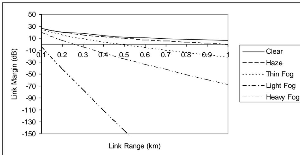
**Fig. (6) Link margin versus link range for 785 nm.**
