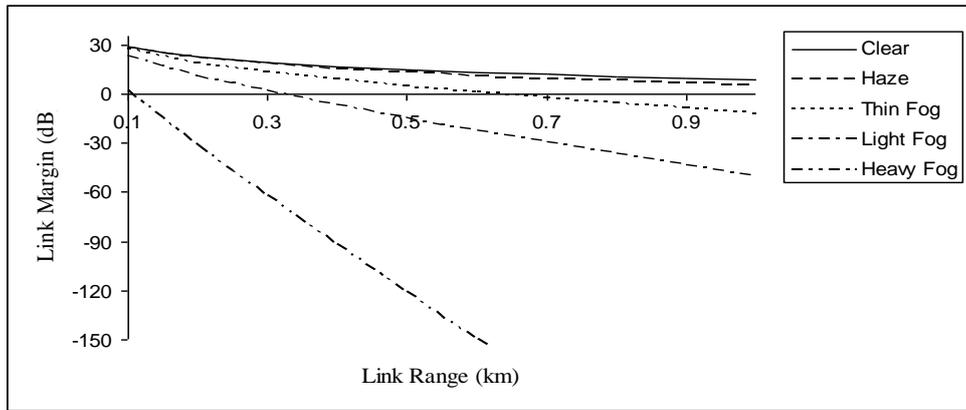
**Fig. (7) Link margin versus link range for 1550 nm.**
