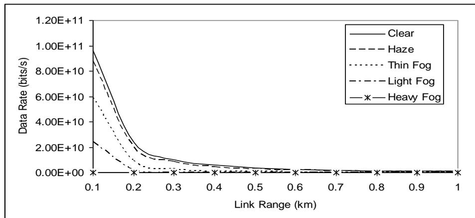
Fig. (10) Data rate versus link range for 1550 nm.
