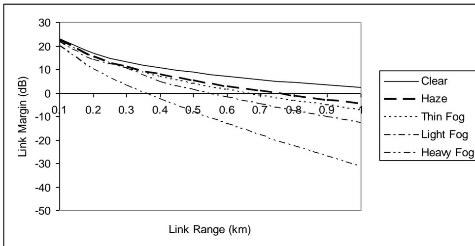
**Fig. (5) Link margin versus link range for 650 nm.**
