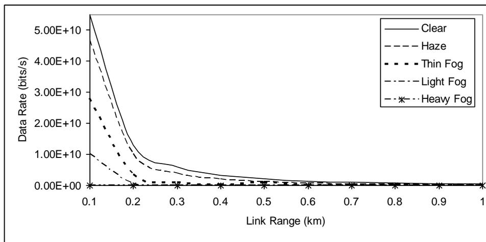
**Fig. (9) Data rate versus link range for 785 nm.**
