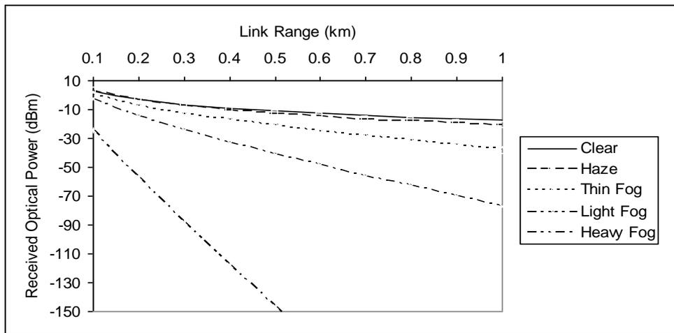
**Fig. (4) Received optical power versus link range for 1550 nm.**
