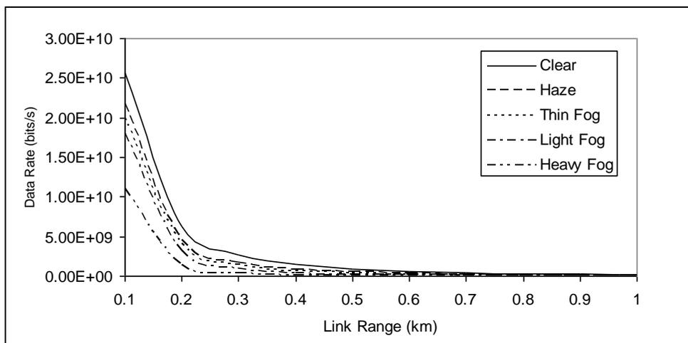
**Fig. (8) Data rate versus link range for 650 nm.**
