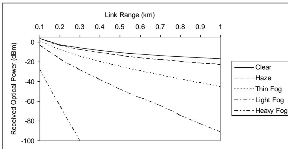
**Fig. (3)** Received optical power versus link range for 785 nm.
