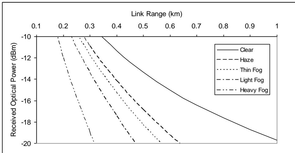
**Fig. (2)** Received optical power versus link range for 650 nm.
