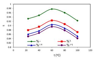
Fig.(5) The variation of exponent s with temperature for Polyester-woven roving fiber E-glass composite.
