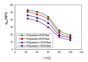
Fig.(3) Ac conductivity of pure Polyester, and doped with different volume fraction of woven roving fiber E-glass, as a function of temperature at constant frequency (400kHz).
