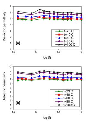
Fig.(1) Variation of dielectric permittivity of: (a)pure Polyester, and (b)19% doped with woven roving fiber E-glass, as a function of frequency at different temperatures.
