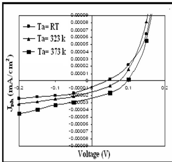
**Fig.(5) I-V characteristics under illumination for PbTe/Si heterojunction at forward and reverse bias voltage at different annealing temperature.**
