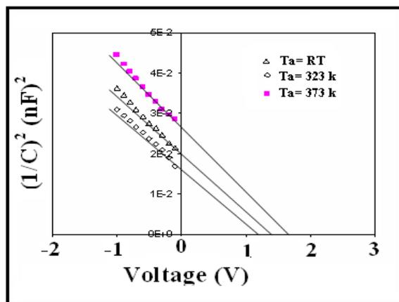
*Fig.(3)  $1/C^2$  as a function of reverse bias voltage and at different annealing temperature.*
