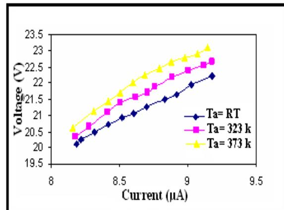
Fig.(2) Variation of Hall voltage versus current for PbTe films at annealing temperatures.
