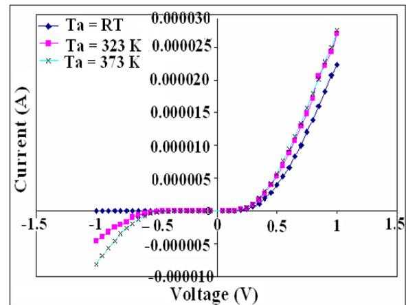
*Fig.(4) I-V characteristics in the dark for PbTe \ Si heterojunction at forward and reverse bias voltage at different annealing temperatures.*
