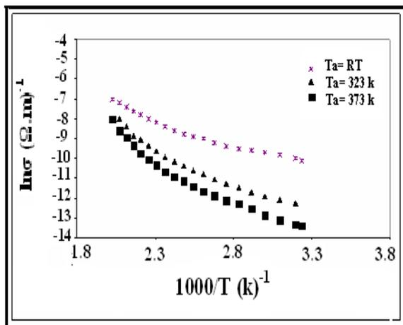
Fig.(1)  $\ln\sigma$  as a function of  $1000/T$  for PbTe films.
