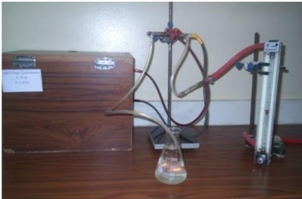
Fig.(2) Ozone generator device with water sample.
