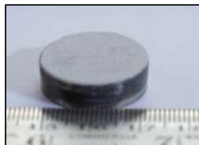
Figure 2. The photograph view of Al-Al 2 O 3 sample with 20 mm diameter.
