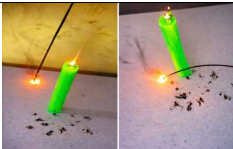
Figure 7: Polycarbonate filament Fire resistance testing for vertical and Horizontal direction
