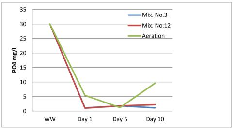
Fig. (4) Removal efficiency of PO<sub>4</sub> in days.
