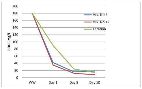
Fig. (2) Removal efficiency of  $BOD_5$  in days.
