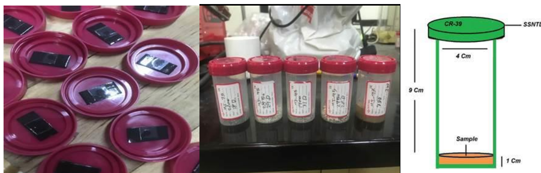
Figure 5. Radon cup technique.
