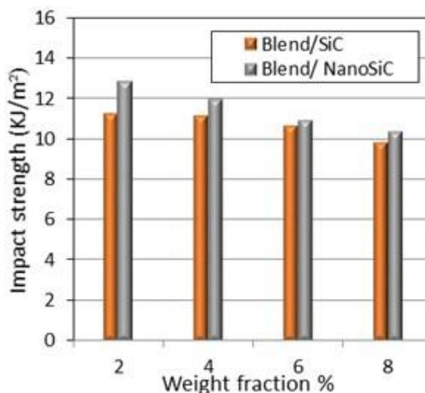
Figure 1: The behavior of impact strength with weight fraction for micro and nano SiC + blend at natural conditions.
