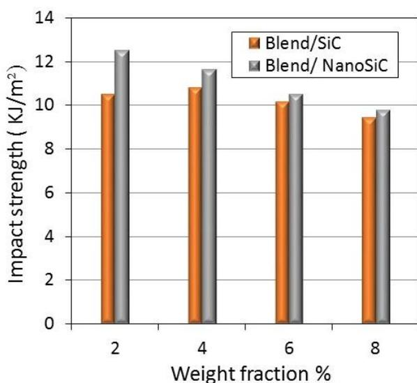
Figure 2: The Impact Strength value relation with weight fraction for particles and nano (SiC + Blend) exposure to UV
