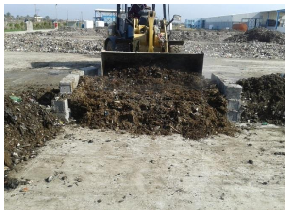
Fig. (1): Pilot scale of the compost piles, including organic fraction of MSW and their treatment with different manure using a windrow system, at the Factory of recycling of organic solid wastes in Al-Usifia City.
