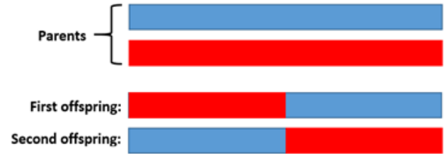
Figure 5. Adopted crossover method for producing the two new offspring.
