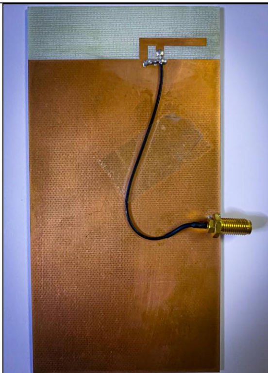
Figure 1. Inverted F-shaped antenna in a cellular phone system.
