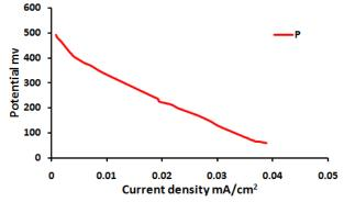
Figure 4. The polarization curve for MFC with the prepared membrane P tested operated after 24 hours cell construction.
