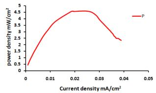
**Figure 5.** The curve of the power density for MFC with prepared membrane *P* tested operated after 24 hours cell construction.
