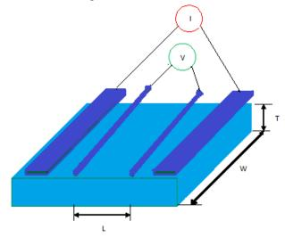
Figure 2. Schematically the membrane electrical contacts in the cell [8].
