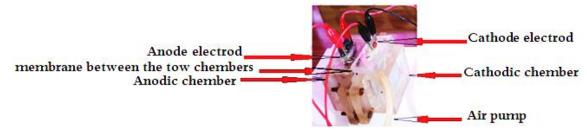
Figure 1. Laboratory Microbial fuel cell.
