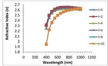
Fig.(5): show that the refractive index as a function of wave length for different time exposure.
