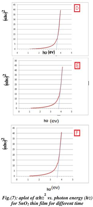
for SnO<sub>2</sub> thin film for different time (A(t=0),B(t=2)min, C(t=4)min, D(t=6)min, E(t=8)min, F(t=10)min).
