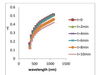
Fig.(3): Transmission spectrum of SnO<sub>2</sub> thin film with wave length for different time
