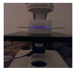
Fig.(1): Photographic picture of DBD system used to treat of films.
