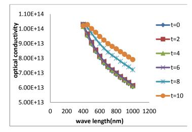
Fig.(8): Optical conductivity as a function of wave length for different time exposure.
