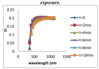
Fig.(4): Reflectance spectrum of SnO<sub>2</sub>thin film with wave length for different time exposure.
