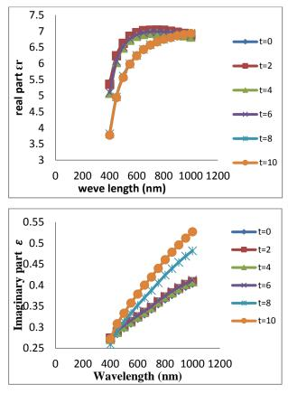
Fig.(4): the real and the imaginary part of dielectric constant SnO<sub>2</sub> different time exposure as function of wavelength.
