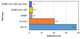
**Figure 6.** Total reflectance values of the selective coatings compared with reflectance from glass mirror and uncoated Al-plate.
