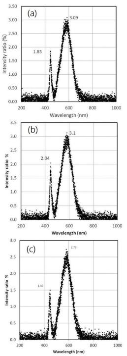
**Figure 5.** The spectral reflectance of the coatings (a) OMBP (b) OMBP with CB (c) OMBP with CBP and LMO.
