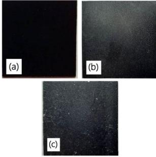
**Figure 1.** The Al-plates coated with different coatings. (a) Commercially available matt black MBP paint (b) MBP air-sprayed with carbon black powder (CBP) (c) MBP air-sprayed with CBP and lithium metal oxide (LMO).
