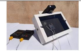
**Figure 3.** The flat-plate collector system used for the measurement of the solar-thermal characteristics.
