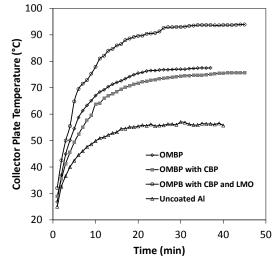
**Figure 7.** The solar-thermal response of the composite coatings as compared with that of the OMBP.
