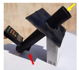
**Figure 2.** A home-made setup for the measurement of total reflection of the solar-radiation. The yellow arrow indicates the entrance of the solar-radiation. The red arrow indicates the specimen location.
