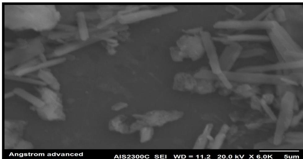
*Fig.(5): SEM image of polyaniline composite PANP.*
