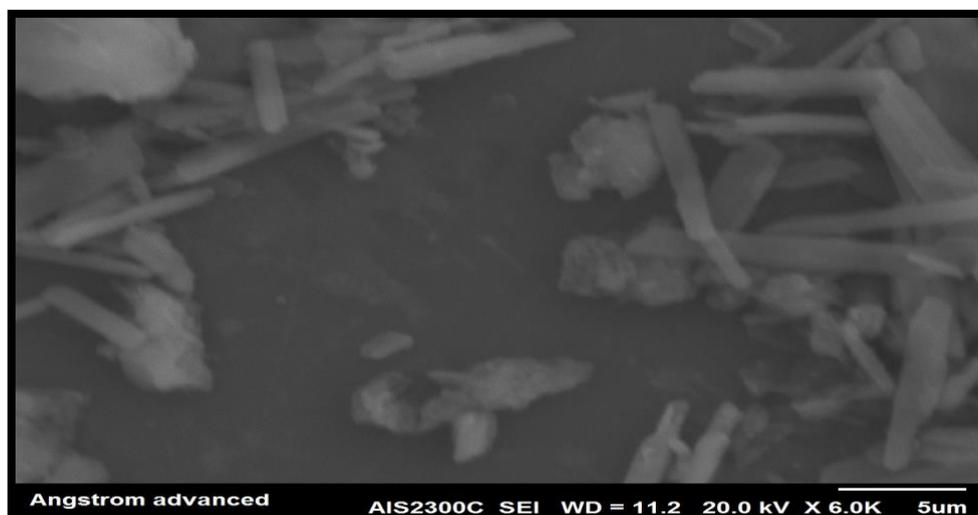
*Fig.(5): SEM image of polyaniline composite PANP.*
