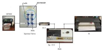
**Scheme 1.** The setup of FIA merging zones system where P: peristaltic pump to flow carrier water, homemade injection valves (in injection status), R. C.: reaction coil, Sp.+F.C: spectrophotometer+ flow cell as detection unit, R.: recorder and drain system.
