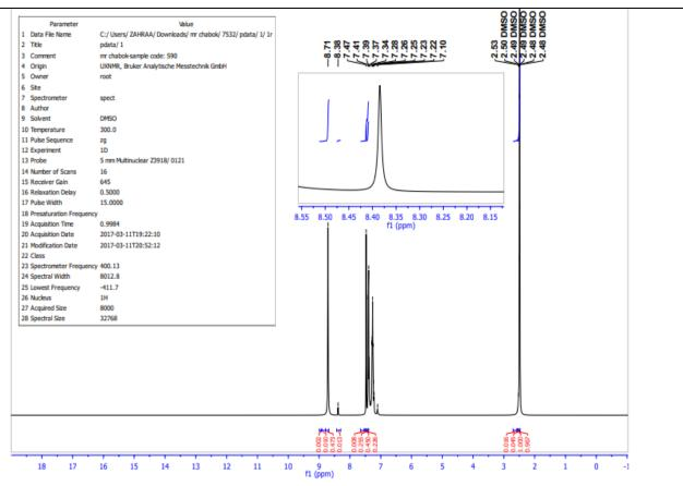
Figure 1. HNMR of 2-(biphenyl-4-yl)-3-((2-(2,4-dinitrophenyl) hydrazono) methyl) imidazo [1,2-a] pyridine (BDNHMIP).
