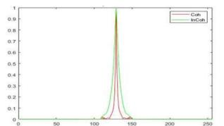
**Figure 7.** The MTF of the Fresnel diffraction in case of incoherent and coherent when R=10 pixels.
