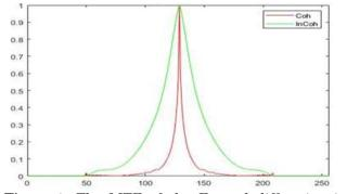
**Figure 8.** The MTF of the Fresnel diffraction in case of incoherent and coherent when R=40 pixels
