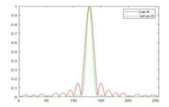
**Figure 1.** The PSF of the Fraunhofer diffraction pattern in case of incoherent and coherent illumination, when R=10 pixels.
