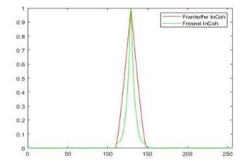
**Figure 11.** The MTF Fresnel Diffraction Pattern and MTF Fraunhofer diffraction, in case of incoherent illumination, when R=10 pixels.
