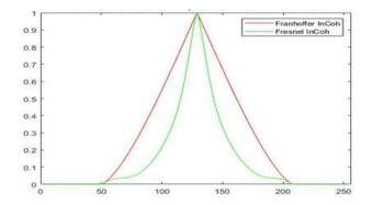
**Figure 12.** The MTF Fresnel Diffraction Pattern and MTF Fraunhofer diffraction Pattern in case of incoherent illumination, when R = 40 pixels.
