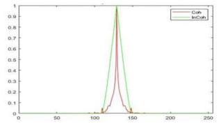
**Figure 3.** The MTF of the Fraunhofer diffraction pattern in case of incoherent and coherent illumination, when R=10 pixels.
