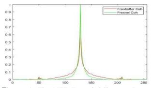
**Figure 10.** The MTF Fresnel diffraction Pattern and MTF Fraunhofer diffraction Pattern, in case of coherent illumination when R=40 pixels.
