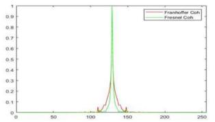
**Figure 9.** The MTF Fresnel Diffraction Pattern and MTF Fraunhofer diffraction, in case of coherent illumination when R=10 pixels.
