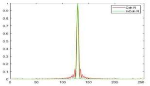
**Figure 2.** The PSF of the Fraunhofer diffraction pattern in case of incoherent and coherent illumination, when R=40 pixels.
