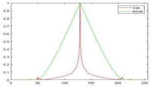
**Figure 4.** The MTF of the Fraunhofer diffraction pattern in case of incoherent and coherent illumination, when R=40 pixels.
