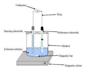
Figure 2. Diagram of ISE cell.
