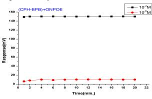
Figure 14. Response time of CPH-ONPOE electrode.
