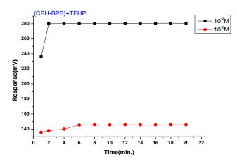
Figure 13. Response time of CPH-TEHP electrode.
