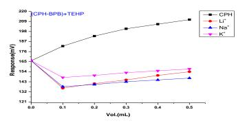
**Figure 15.** Selectivity for CPH-TEHP for mono-cations by match potential method.
