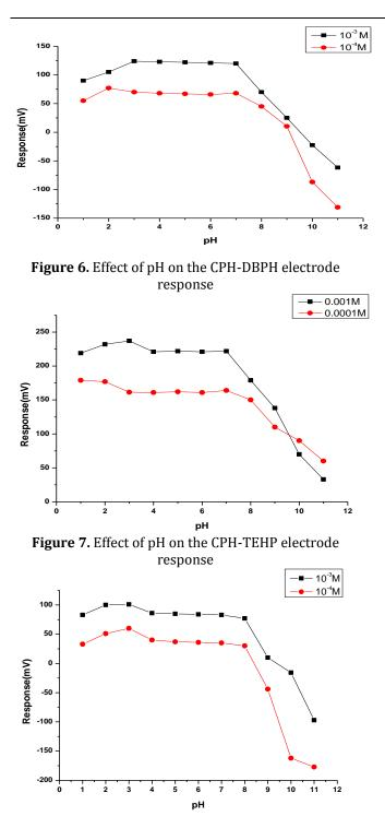
Figure 8. Effect of pH on the CPH-ONPOE electrode response
