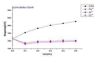
Figure 17. Selectivity for CPH-TEHP for tri-cations by match potential method.
