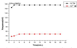
Figure 12. Response time of CPH-DBPH electrode.
