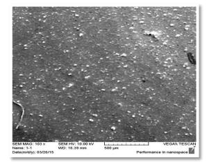
Fig.(2): SEM, Analysis Ag nanoparticles synthesis by of the N. oleander.
