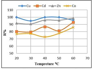
Fig.(11): Effect of the temperature of solution on metal ions removal by polymer  $P_2$ .
