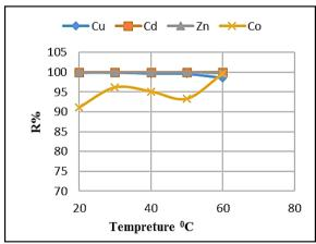
Fig.(10): Effect of the temperature of solution on metal ions removal by polymer  $P_{I}$ .
