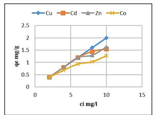
Fig.(8): Effect of initial metal ion concentration on metal ions removal by polymer  $P_1$ .
