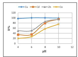
Fig.(6): Effect of the pH of solution on metal ions removal by polymer P<sub>2</sub>.
