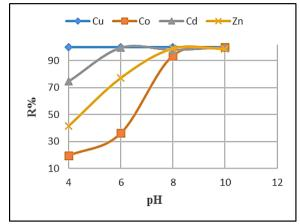
Fig.(5): Effect of the pH of solution on metal ions removal by polymer  $P_1$ .
