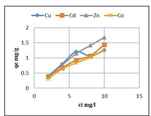
Fig.(9): Effect of initial metal ion concentration on metal ions removal by polymer P<sub>2</sub>.
