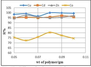
Fig.(7): Effect of polymer weight onto metal ions removal by polymer 2.
