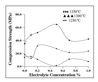
Figure(4). The Compressive Strength for different concentration of electrolyte solution as a function of sintering temperatures.
