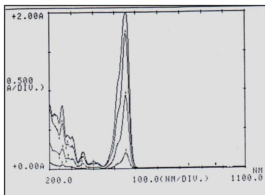
**Fig.(1) : UV-Visible absorption spectrum for dyes solutions with concentration ranging (1-20) mgL<sup>-1</sup>.**
