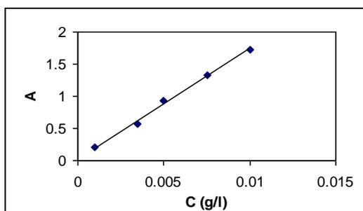
**Fig. (2): Calibration curve of adsorption Rhodamine B dye at (λ<sub>max</sub>=554).**
