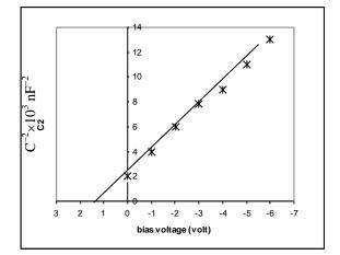
Fig.(5) :  $C^{-2}$  versus Bias voltage for characteristics SnO<sub>2</sub>/InP heterojunction.
