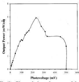
Fig.(9) : Photovoltaic performance of the cell.
