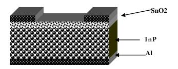
Fig.(1) : Cross-sectional view of heterojunction.
