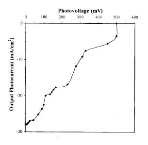
Fig.(8) : Illuminated J-V characteristics of the fabricated cell.
