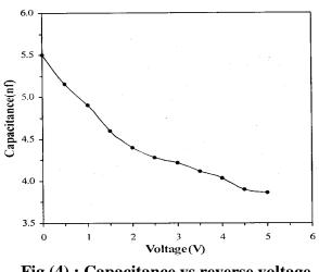
Fig.(4) : Capacitance vs reverse voltage curve.
