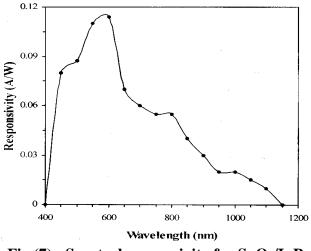
Fig.(7) : Spectral responsivity for SnO<sub>2</sub>/InP.
