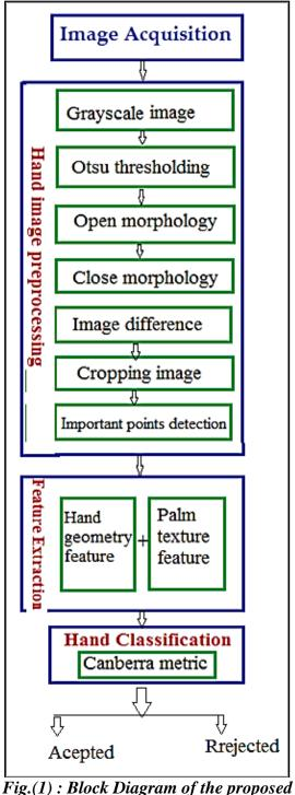
Fig.(1) : Block Diagram of the proposed system.
