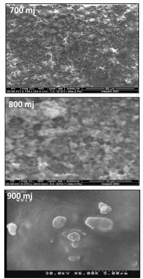
Fig.(4): FESEM images of ZnO NPs prepared by pulsed laser ablation in ethanol with different energyies (700, 800, 900 m.J) and pulses fixed (2000).
