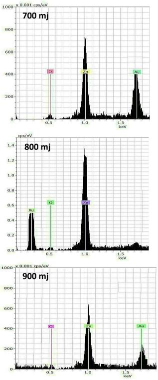
Fig.(5): EDX of ZnO thin films deposited on a glss substrate at 85 C for ethanol with different laser energies (700, 800 and 900 mJ).
