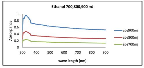
Fig.(6): Optical absorption as a function of wavelength for ZnO prepared on glass substrate with laser pulses of 2000 at different laser energies of (700,800,900 mJ).
