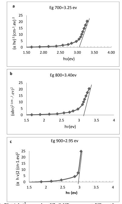
Fig.(7): Plot (ahv)<sup>2</sup> versus hv of ZnO NPs prepare at different laser energies (a) 700 (b)800 (c) 900mJ.
