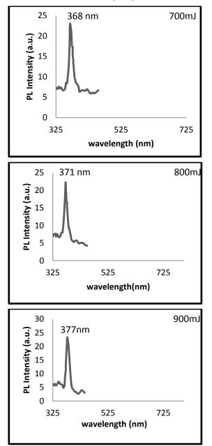
Fig.(8): PL spectra of ZnO NPs prepared at differences laser energies.
