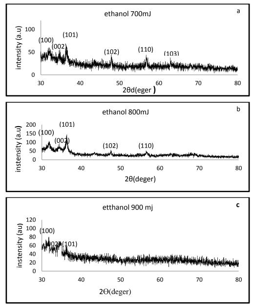
Fig. (3) : XRD pattern of ZnO NPs with different energies (a) 700mJ(b) 800 mJ and (c) 900mJ on glass substrate at 2000 puls.
