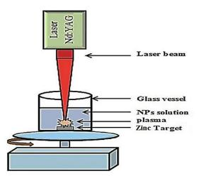
Fig.(1): Experimental setup of noanoparticles synthesis by PLA method.
