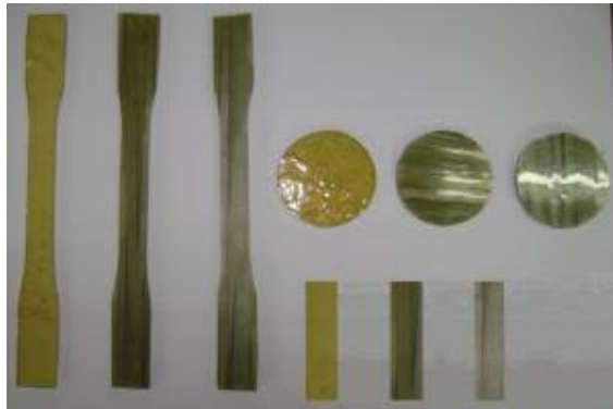
Fig. (3) : Form of the test requirements for thermal conductivity, impact and tensile tests.
