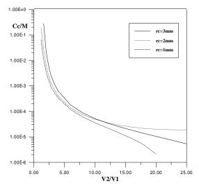
Fig.(11) : The relative chromatic aberration coefficient  $C_c/M$  as a function of the voltage ratio V2/V1 at various values of the electrode radius  $r_c$ .
