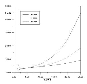
Fig.(7): The relative chromatic aberration coefficient  $C_c/f_i$  as a function of the voltage ratio V2/V1 at various values of the electrode radius  $r_c$ .
