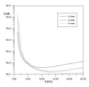
Fig.(6) : The relative spherical aberration coefficient  $C_s/f_i$  as a function of the voltage ratio V2/V1 at various values of the electrode radius  $r_c$ .
