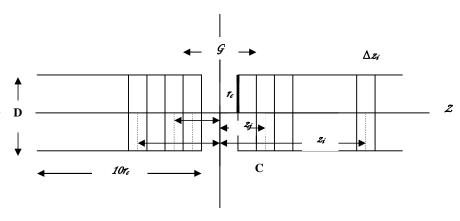
Fig.(2) : Simple coaxial two-cylinder lens consisting of a large number of circular strips in order to obtain the potential distribution by CDM.
