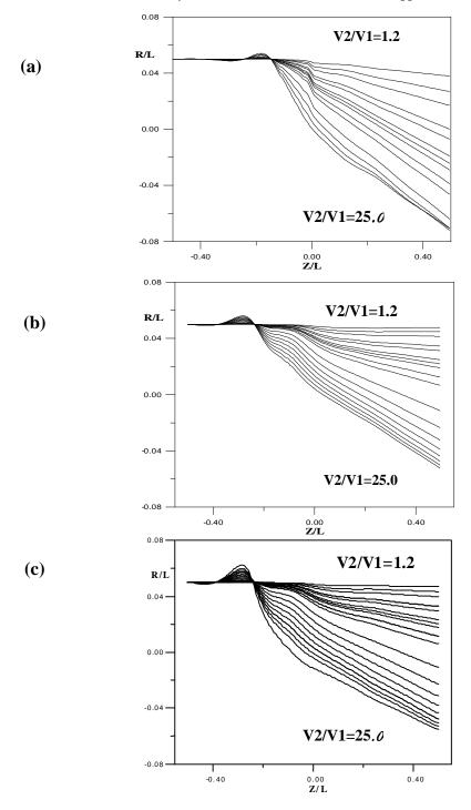
Fig.(5): The electron beam trajectory in an electrostatic lens under zero magnification condition at various values of the electrode radius  $r_c$  (a) 1 mm (b) 2 mm (c) 3 mm for a wide range of the voltage ratio (V2/V1 = 1.2, 1.4, 1.6, 1.8, 2.0, 2.2, 2.4, 3.0, 3.5, 4.0, 6.0, 8.0, 10.0, 16.0, 18.0, 20 and 25.0).
