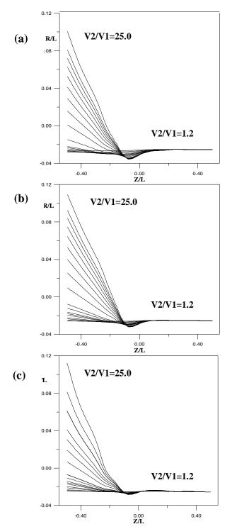
Fig.(9): The electron beam trajectory in an electrostatic lens under finite magnification condition at various values of the electrode radius  $r_c$  (a) 1 mm (b) 2 mm (c) 3 mm for a wide range of the voltage ratio (V2/V1 = 1.2, 1.4, 1.6, 1.8, 2.0, 2.2, 2.4, 3.0, 3.5, 4.0, 6.0, 8.0, 10.0, 16.0, 18.0, 20.0, and 25.0).
