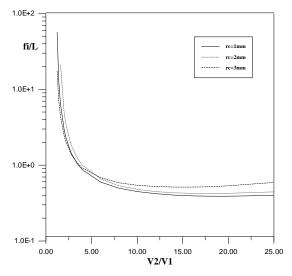
Fig.(8) : The relative image-side focal length  $f_i/L$  as a function of voltage ratio V2/V1 at various values of the electrode radius  $r_c$  under zero magnification conditions.
