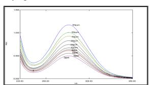
Fig.(8) Spectra for CPSS solutions at different concentration ranged from 2-64 mg/L.
