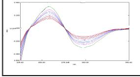
Fig.(9) The first derivative spectra for CPSS solutions 2-64 mg/L.
