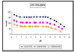
Fig.(4) Effect of pH on the potential of the electrode A1 at concentrations  $10^{-2}$ ,  $10^{-3}$  and  $10^{-4}$  M.
