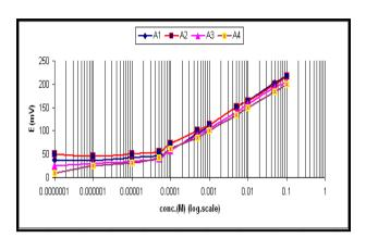
Fig.(3) Calibration curves of Chloramphenicol sodium succinate selective electrodes using DBPH, DPB, DOP and TBP plasticizer.
