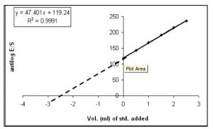
Fig.(6) Plot of antilog (E/S) versus the volume of chloramphenicol sodium succinate using A1 electrode.
