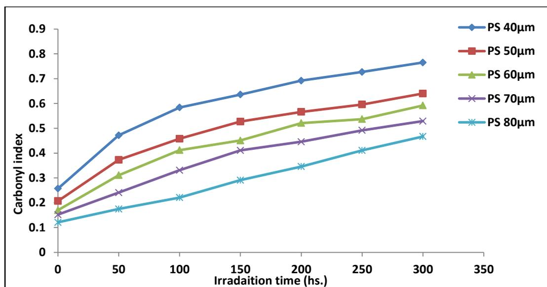
Fig.(2): Relationship between ( $I_{CO}$ ) and irradiation time for PS blank films in different thicknesses.
