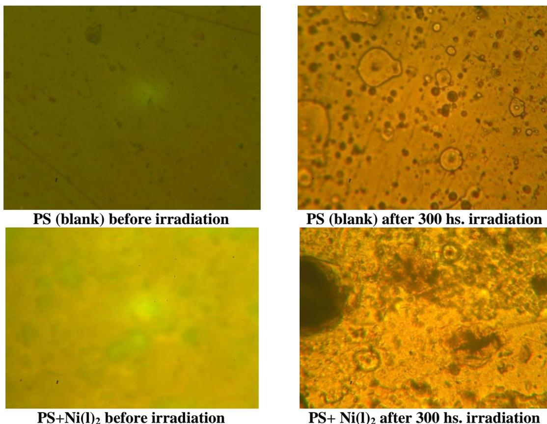
*Fig.(17): Microscopic images of PS(blank) and PS+Ni(L)<sub>2</sub>.*
