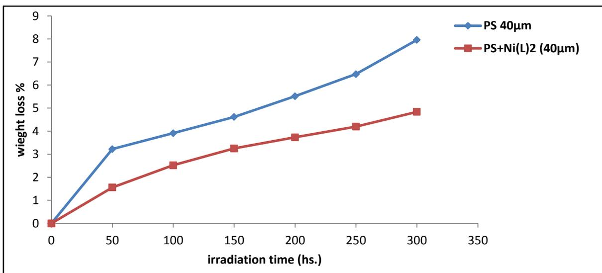
Fig.(12): Loss in weight(%) vs. irradiation time for PS blank and PS+Ni(L)<sub>2</sub> films in 40µm thickness.
