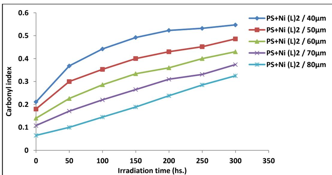
Fig.(3): Relation between ( $I_{CO}$ ) and irradiation time for PS+Ni(L)<sub>2</sub> in different thicknesses.
