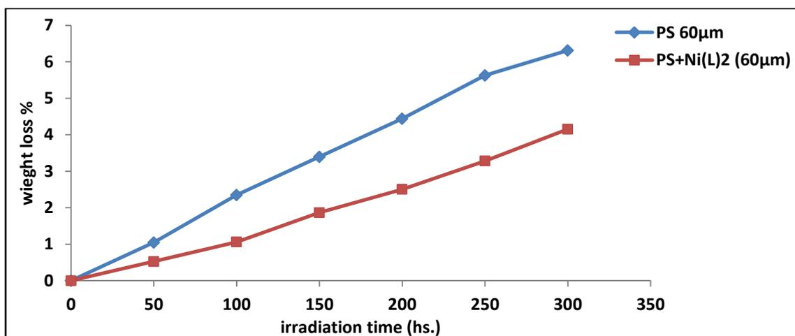
Fig.(14): Loss in weight(%) vs. irradiation time for PS blank and PS+Ni(L)<sub>2</sub> films in 60 µm thickness.
