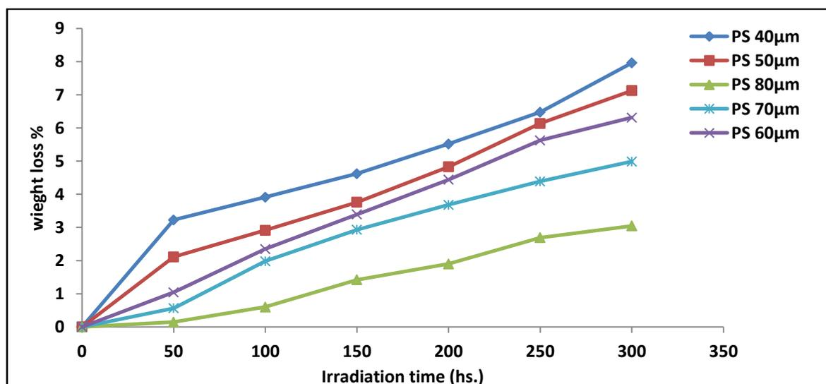
*Fig.(10): Loss in weight (%) vs. irradiation time for PS blank films in different thickness.*
