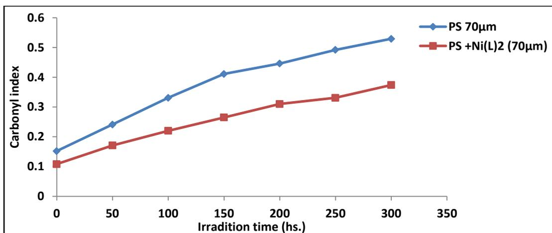
Fig. (7): The relationship between ( $I_{CO}$ ) and irradiation time for PS (blank) and PS+Ni(L)<sub>2</sub> in 70µm thickness.
