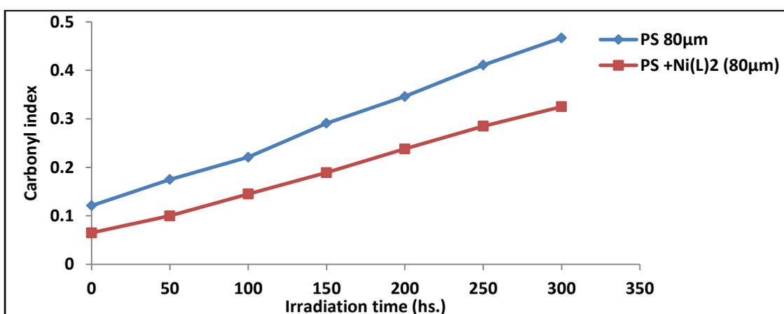
Fig. (8): The relationship between ( $I_{CO}$ ) and irradiation time for PS (blank) and PS+Ni(L)<sub>2</sub> in 80µm thickness.
