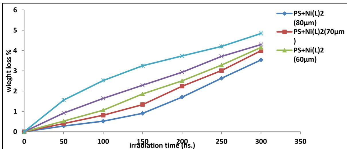
Fig.(11): Loss in weight(%) vs. irradiation time for PS+Ni(L)<sub>2</sub> films in different thickness.
