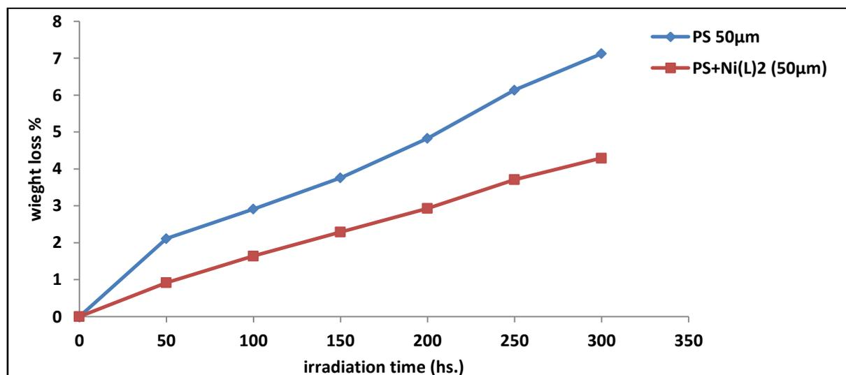
Fig.(13): Loss in weight(%) vs. irradiation time for PS blank and PS+Ni(L)<sub>2</sub> films in 50µm thickness.
