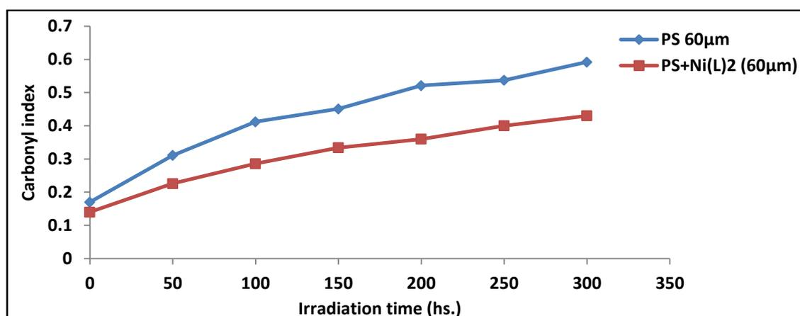
Fig.(6): The relation between ( $I_{CO}$ ) and irradiation time for PS (blank) and PS+Ni(L)<sub>2</sub> in 60µm thickness.
