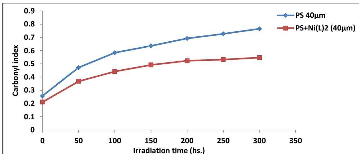
Fig.(4): The relation between ( $I_{CO}$ ) and irradiation time for PS (blank) and PS+Ni(L)<sub>2</sub> in 40µm thickness.
