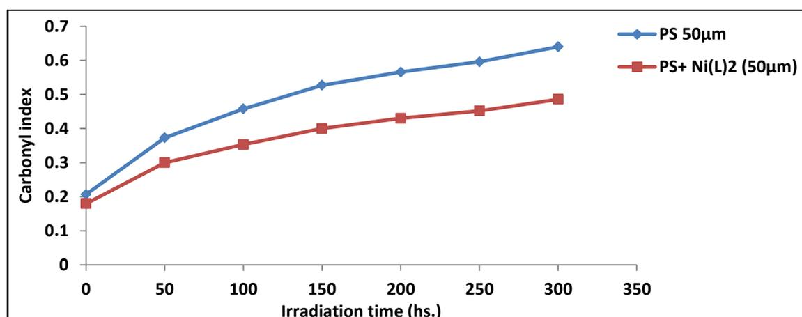
Fig.(5): The relation between ( $I_{CO}$ ) and irradiation time for PS (blank) and PS+Ni(L)<sub>2</sub> in 50µm thickness.
