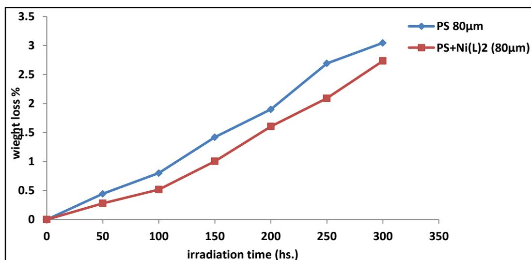
Fig.(16): Loss in weight(%) vs. irradiation time for PS blank and PS+Ni(L)<sub>2</sub> films in 80 µm thickness.
