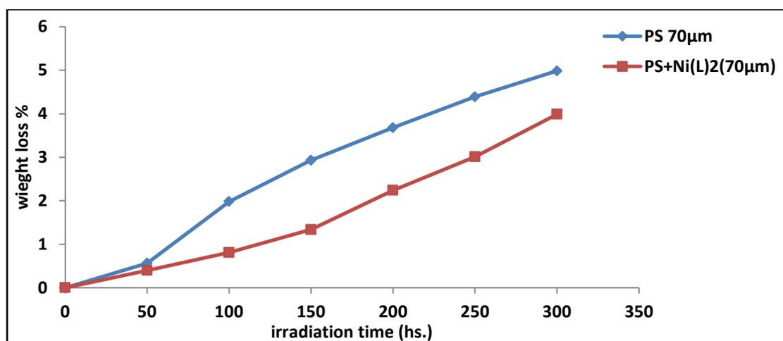
Fig.(15): Loss in weight(%) vs. irradiation time for PS blank and PS+Ni(L)<sub>2</sub> films in 70 µm thickness.
