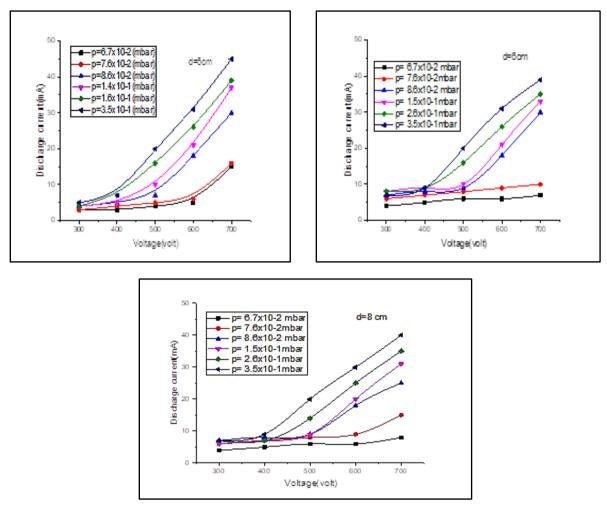
Fig.(3): Discharge current as function of voltage at different pressures of Ar gas for different electrodes separation using V target.
