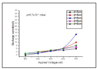
Fig.(4): Variation of discharge current with a voltage at differed electrodes separation of Ar gas for V target.
