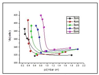
Fig.(5): Paschen curves of the Ar gas discharge plasma at different electrodes separation.
