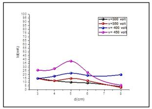
Fig.(8): Variation of discharge current with inter-electrode distance at certain discharge voltages without using a magnetron.
