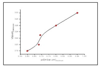
Fig.(6): Minimum values of breakdown voltage as a function of electrodes separation.
