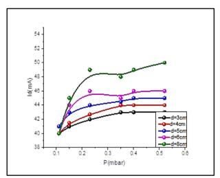
Fig.(7): Variation of discharge current with pressure at different electrodes separation.
