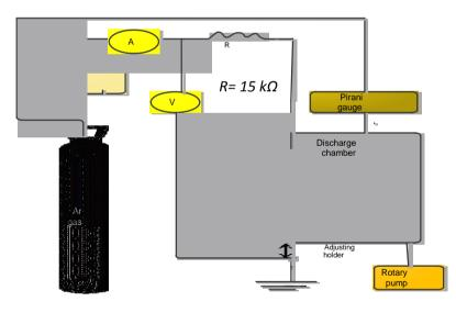
Fig.(2): Dc-glow discharge plasma set-up.
