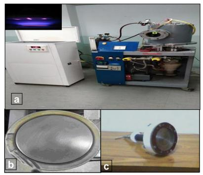
Fig.(1): A Photographic of the major experimental set-up utilized in this work. (a) Plasma Chamber cell (b) anode electrode (c) cathod electrode.
